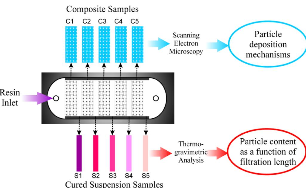
Figure 1: Experimental set up for the infiltration tests
