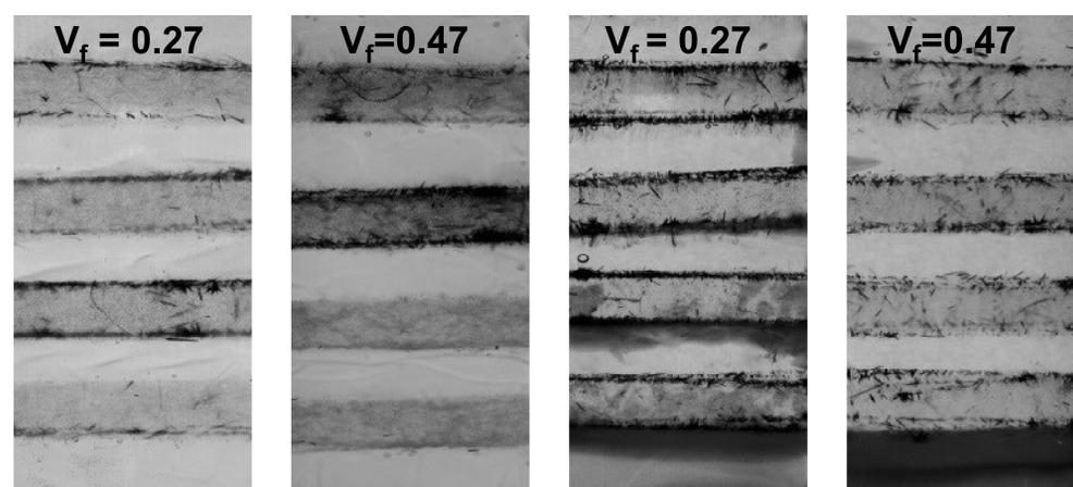
Figure 4: Visual observation of the cured composites. The inlet is located at the bottom of each picture.
